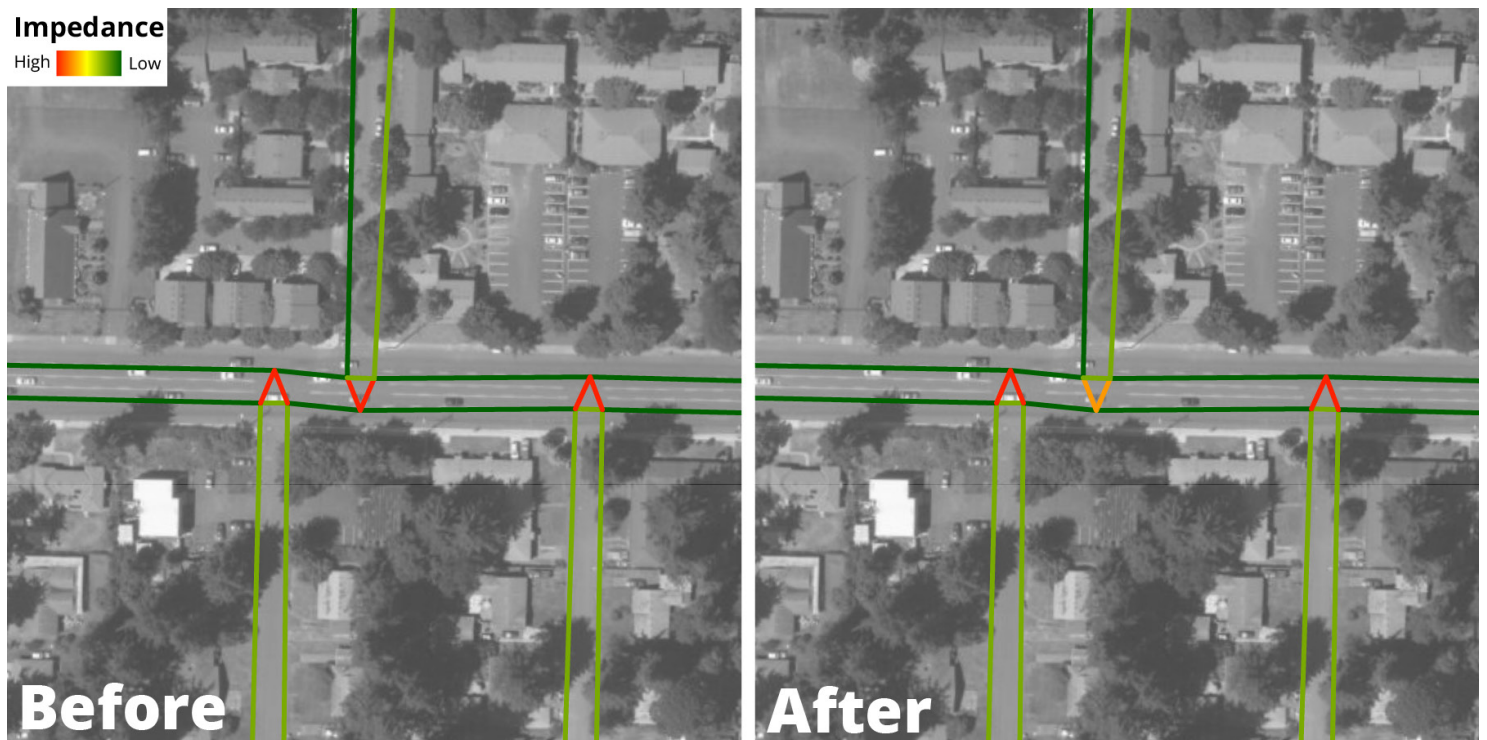
The example above shows the network before and after a crossing projects at Stark Street and 136th Avenue. Notice how the impedance decreases with the introduction of a Rectangular Rapid Flash Beacon (RRFB).
